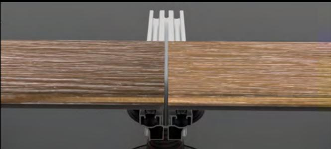
Compulsory 4mm expansion gap and 4 spacers at all short ends. Do not use spacers in all joists.
